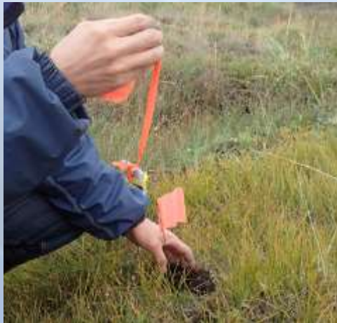
Measuring near-surface soil temperature (Tnss)
