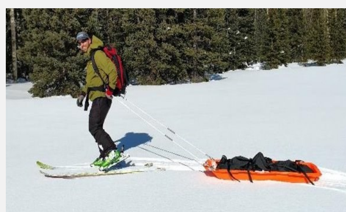
Figure 1. GPR sled being towed by R. Webb during SnowEx 2017 on Grand Mesa, CO.
