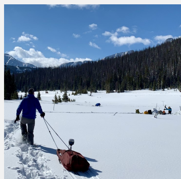
Figure 4. GPR sled being pulled by R. Bonnell during SnowEx 2020 at Cameron Pass, CO.
