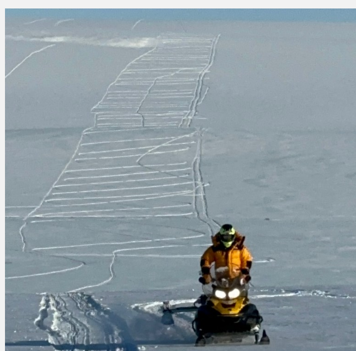
Figure 3. GPR mounted on T. Meehan's snowmobile during SnowEx 2023 in Alaska.
