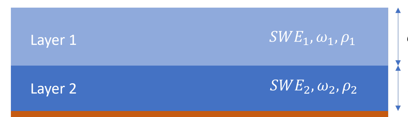
Figure 2: Two-layer model for SWE retrieval. Layer 1 and layer 2 consists of individual parameters of SWE, \omega and density.
