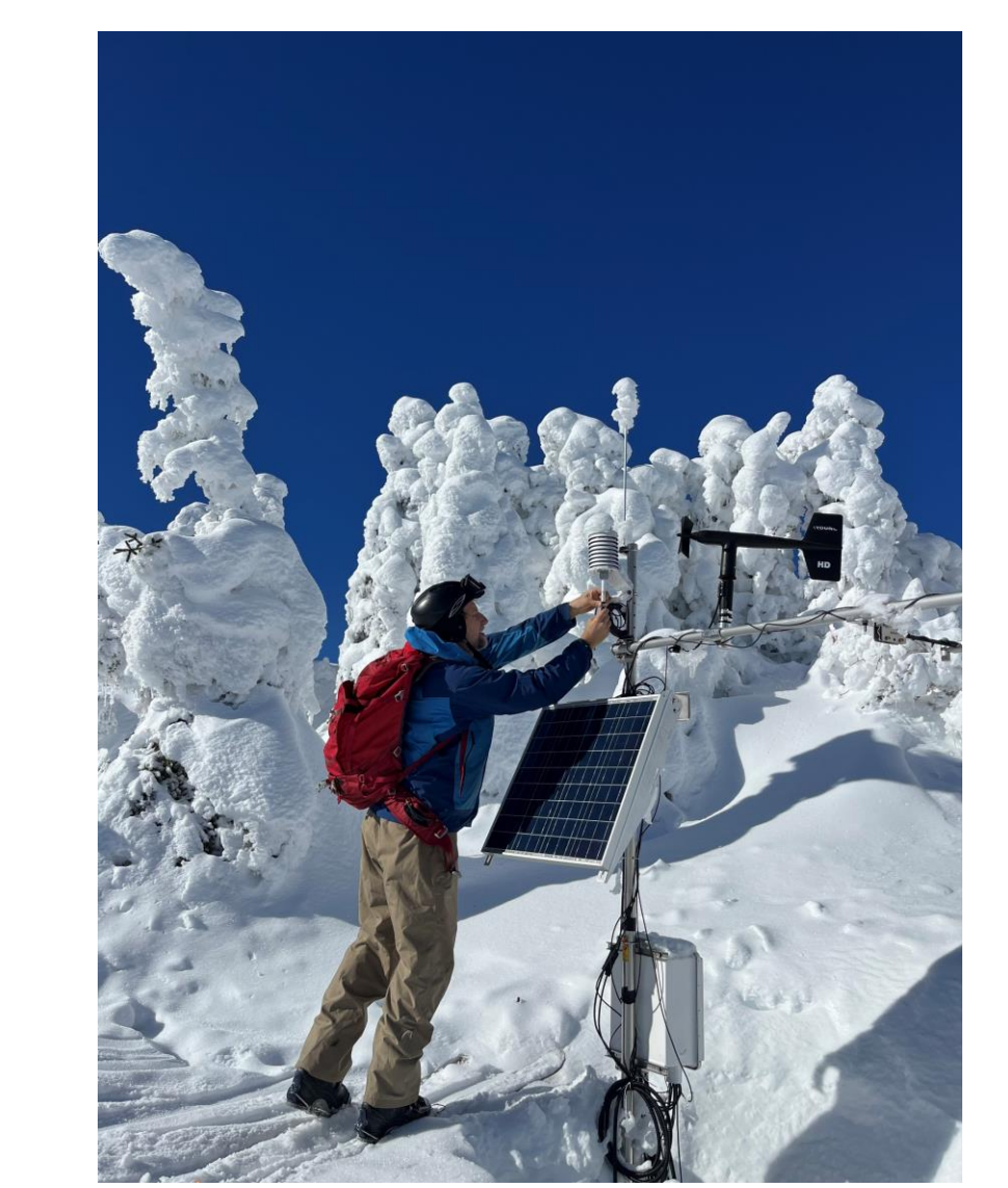
Fig. 6: Maintenance at the summit (SUMM) S2S meteorology and snowpack monitoring site.
