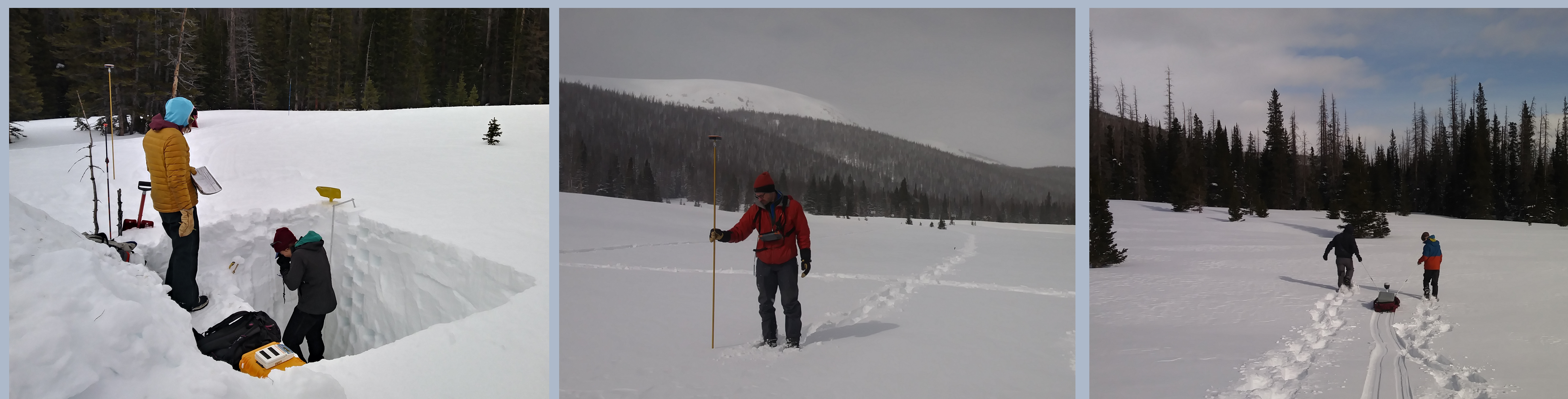
Photos of COCPJW snowpit observations, manual probing along Meadow Transect, and GPR survey along North Transect.
