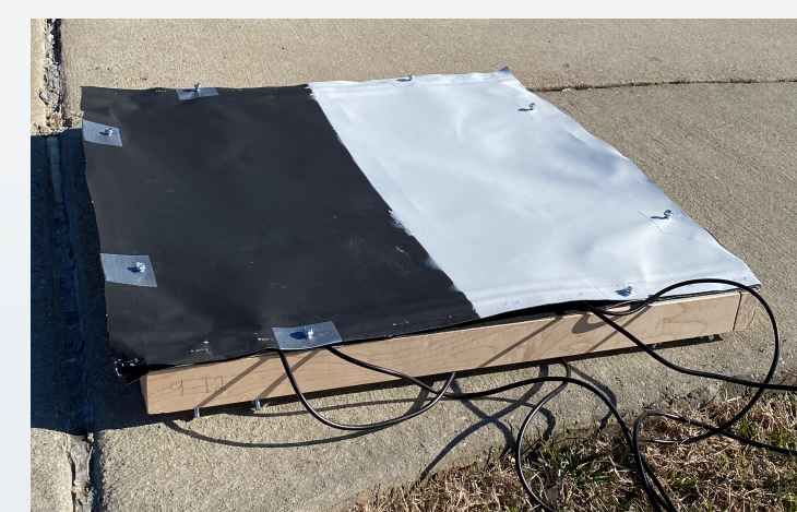
Calibration Target (+/- 0.5 °C accuracy)
