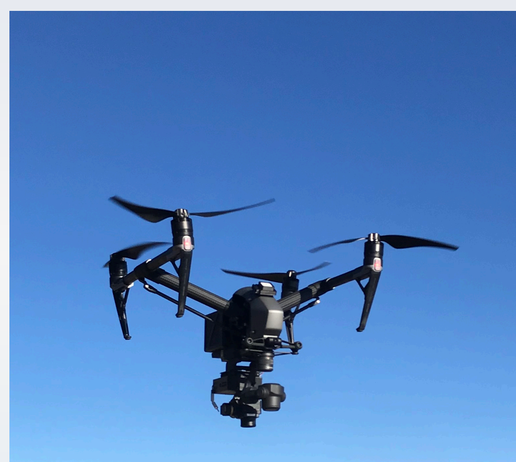
DJI Inspire 2 – Dual Gimbal-Mounted Thermal and RGB Cameras
