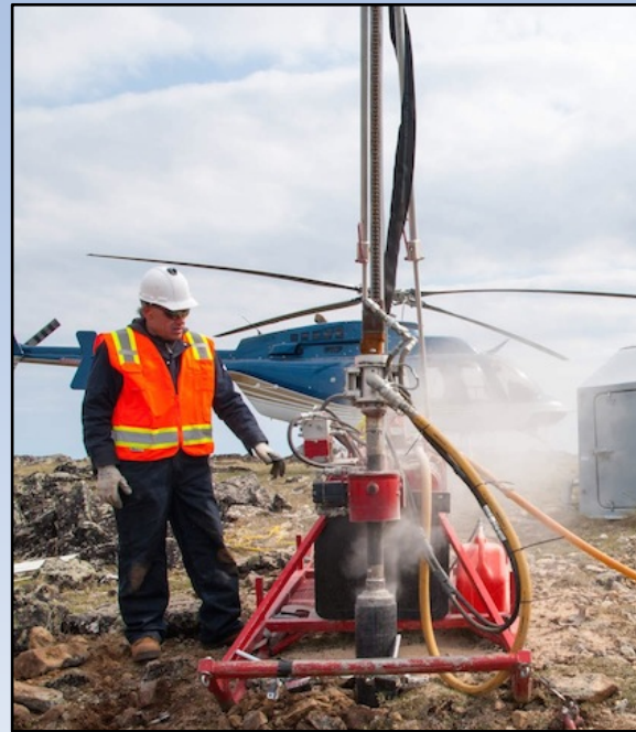
Sensor is installed in a borehole 1 – 5 m deep
