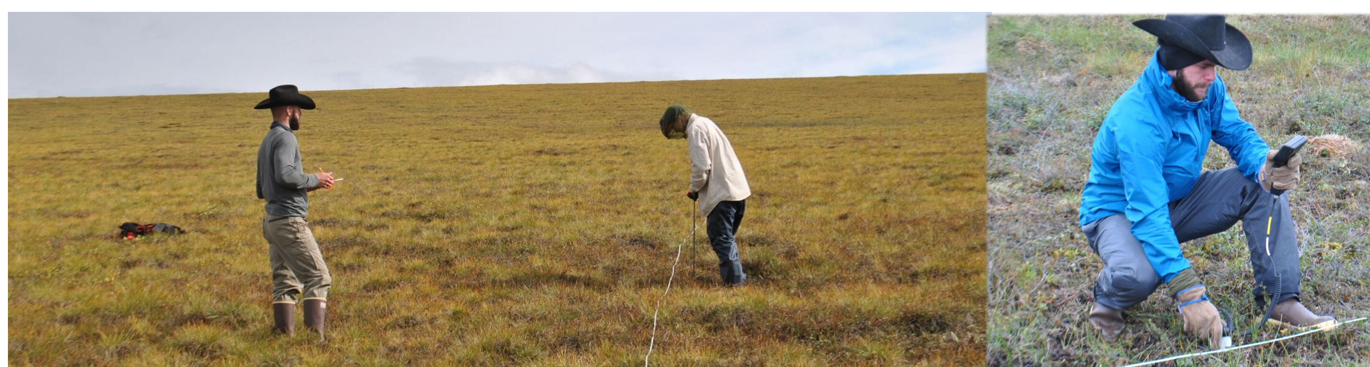
Figure 3: Measuring ALT on North Ridge using active layer probe. Right: Collecting soil moisture data using hand-held HydroSense II soil moisture probe.
