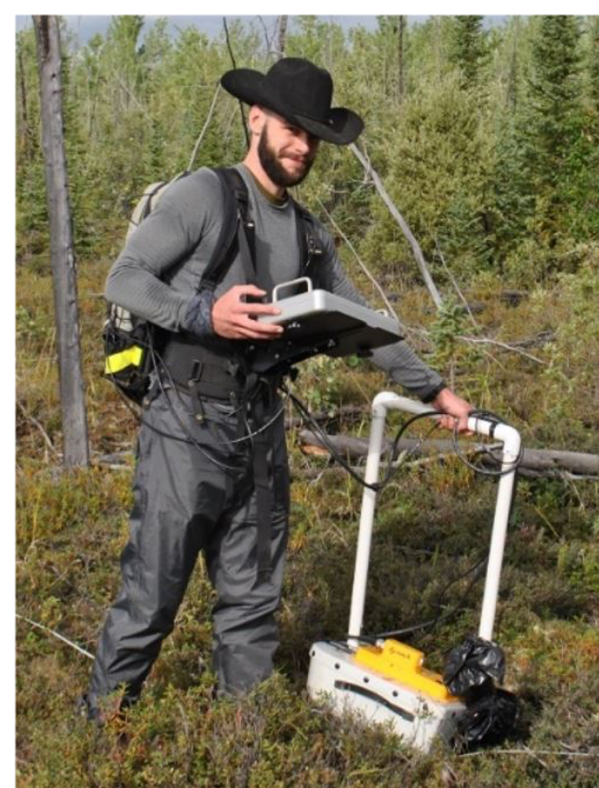
Figure 5: Shows the GPR with handle in use. The control unit and monitor are attached to the backpack, and the 500MHz antenna is attached to the handle. August 2017 Photo from survey line near Delta Junction, AK.
